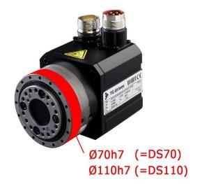
In case of centering of rotating part which is mounted on actuator reducer is recommended to center this part on inner diameter of cycloidal reducer which is tolerated. On some types of DriveSpin rotary actuators is an inserted sealing in this diameter, which can be moved deeper into the body of reducer by simple tapping.
